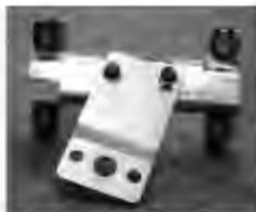
Attach drop bracket to 4wd-linkage, using the factory bolts and washers that are included in the body lift kit.
