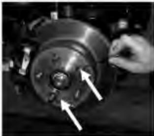
TIP: If you install aftermarket wheels, you must remove rotor retainers (2 on each wheel) to allow aftermarket wheel to sit flat on rotor. - Wire snips
