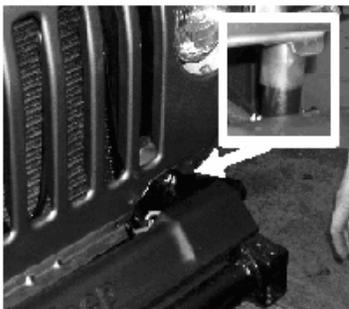
Replace factory bump stops with bumps - swivel 13mm socket stops from Body lift kit with the rounded side pointing downwards. Tighten bolts (you might need to lift the vehicle to get access to the bolts). Repeat on other side of the vehicle.
