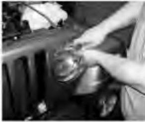
Light bezels must be removed to install new bump stops with the 3" body lift - T-15 screw driver
